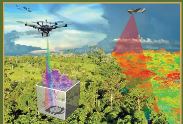
Different remote sensing approaches (airplane and drone Lidar scanning, orbital sensors, and machine learning) to monitor forest restoration. Image: Daniel Papa
